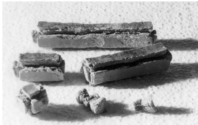
Fig. 8 Samples of SSC95–100S after storage in MgSO_4 solution
